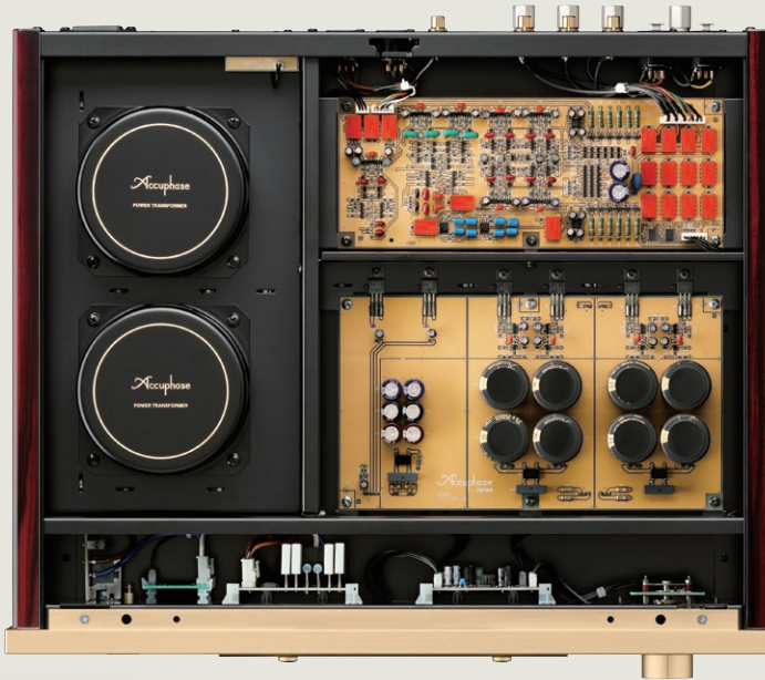
Internal layout realizes full mono construction to prevent mutual interference between channels
